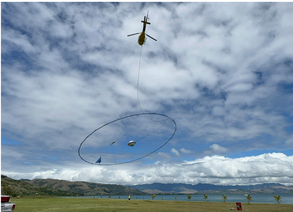
Airborne Electromagnetic (AEM) equipped helicopters help in the surveys of Viti Levu. Photo: SUPPLIED
